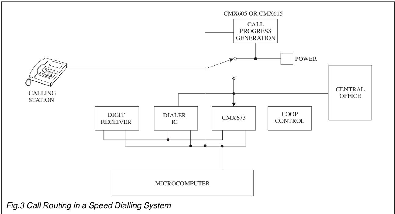
Fig.3 Call Routing in a Speed Dialling System
