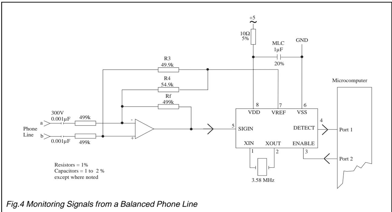
Fig.4 Monitoring Signals from a Balanced Phone Line
